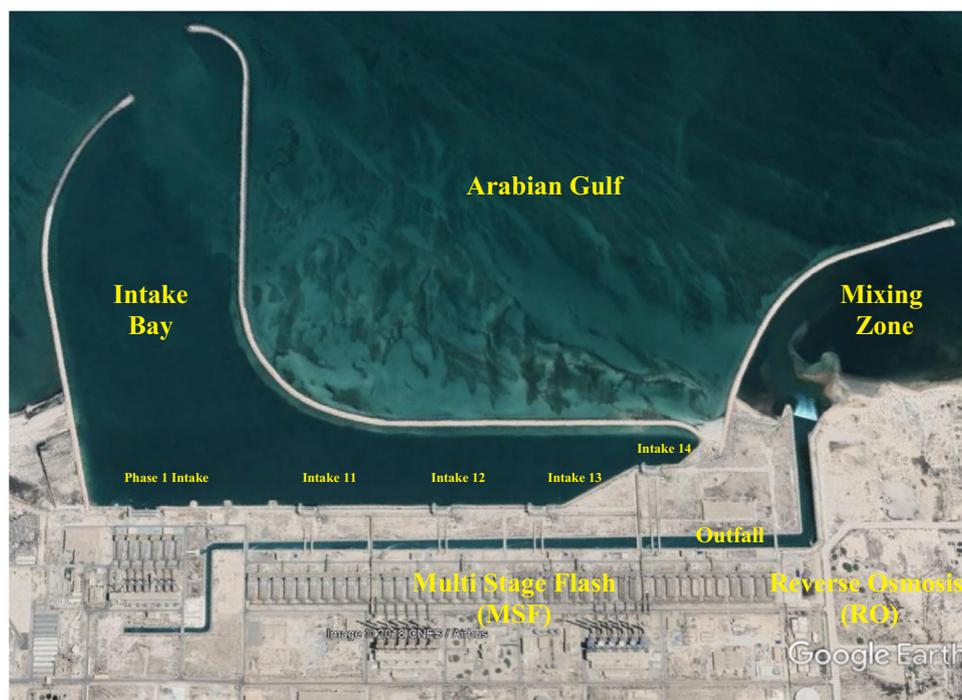
Fig. 1. Satellite view of the coastal area of the Jubail desalination and power plants showing: intake bay, outfall and mixing zone. (<https://earth.google.com/web/>).
